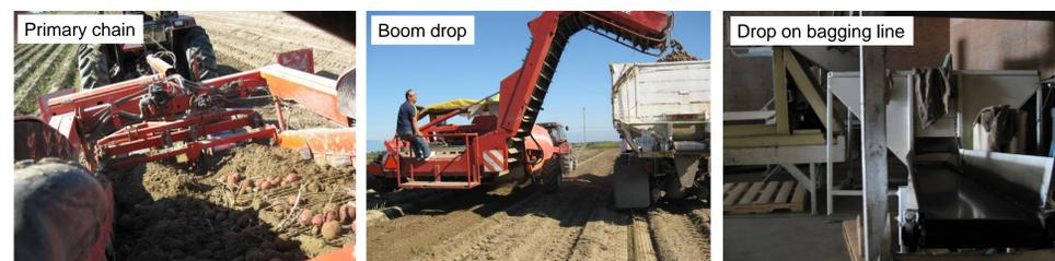
Figure 3. Locations that appear to be critical in causing damage at harvest
